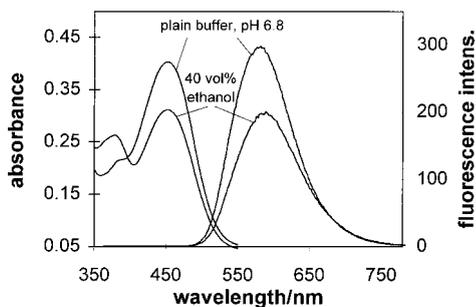
**Fig. 6** Absorbance and fluorescence spectra of the ethanol sensor layer ( $\text{ETH}^{\text{T}} 4004$ , 20 mol% tridodecylammonium chloride (TDMACl) relative to the reactand, PVC, DOS) in contact with a plain buffer and 40 vol% of ethanol, showing the decrease in absorbance and fluorescence emission of the trifluoroacetyl form and the increase in absorbance of the hemiacetal.
