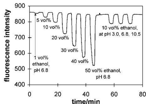
**Fig. 7** Response curve of the ethanol sensor layer ( $\text{ETH}^{\text{T}} 4004$ , 20 mol% TDMACl relative to the reactand, PVC, DOS) on exposure to aqueous ethanol solutions. The excitation and emission wavelengths were set to 450 and 560 nm, respectively.
