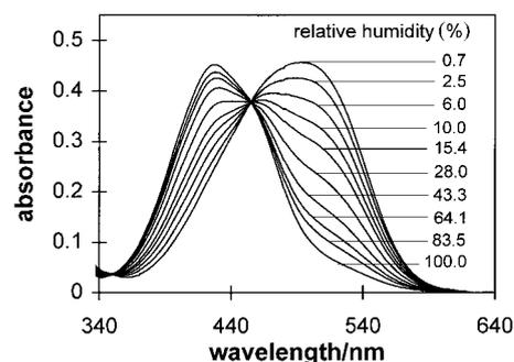
**Fig. 8** Absorbance spectra of the humidity-sensitive layer ( $\text{ETH}^{\text{T}} 4001$ , 20 mol% TDMACl relative to the reactand, polyurethane Tecoflex) in contact with different concentrations of humid air. When changing from dry to humid air, the trifluoroacetyl group of the reactand  $\text{ETH}^{\text{T}} 4001$  is converted into a diol. The chemical reaction is fully reversible.
