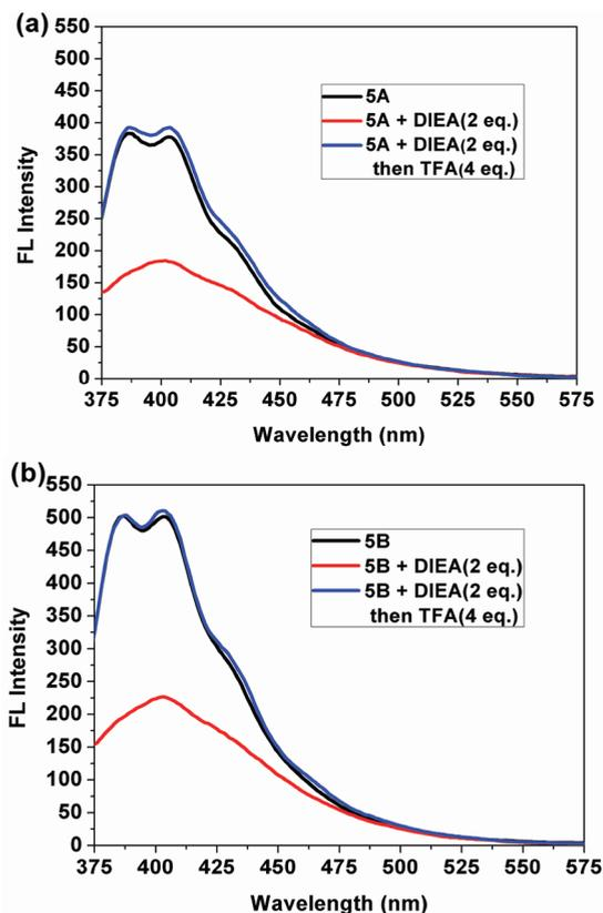
**Figure 4.** Fluorescence spectra of [2]catenanes **5A** and **5B** ( $\lambda_{exc} = 356$  nm,  $1 \times 10^{-5}$  M, 298 K) in  $\text{CH}_3\text{CN}$  before deprotonation (black), after deprotonation with 2 equiv of DIEA (red), and reprotonation with 4 equiv of trifluoroacetic acid (TFA, blue).
