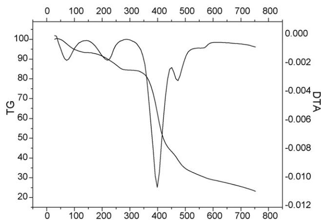
Fig. 6. TG and DTA curves for original Eu(III) complex.
