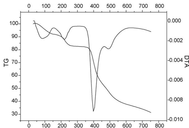
Fig. 8. TG and DTA curves for original Gd(III) complex.
