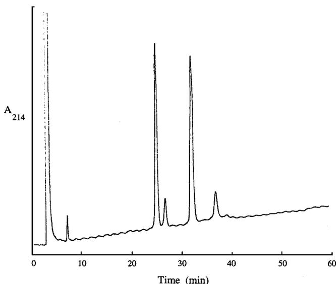
Figure 1. Analysis of brown antechinus glutathione transferase subunits by reverse-phase hplc. An aliquot (100  $\mu$ l) of the acidic fraction obtained after affinity chromatography of pooled male cytosol was injected onto the hplc column (7  $\mu$ m, C<sub>18</sub> reverse-phase) under the conditions described in the Materials and methods section. When similar samples obtained from female animals were analysed, a clear sex-difference in the GST isoenzyme profile was not observed.
