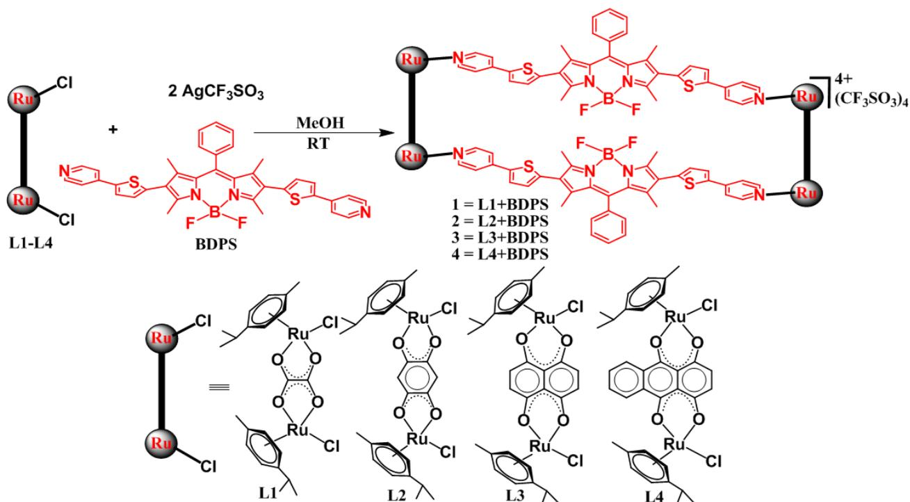
**Scheme 1.** Reaction scheme for the synthesis of metalla-rectangles 1-4.
