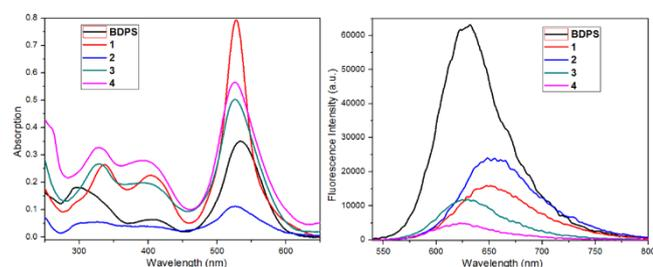
**Figure 2.** Absorption (left) and emission (right) spectra of BDPS and rectangles **1-4** in  $\text{CH}_2\text{Cl}_2$ .
