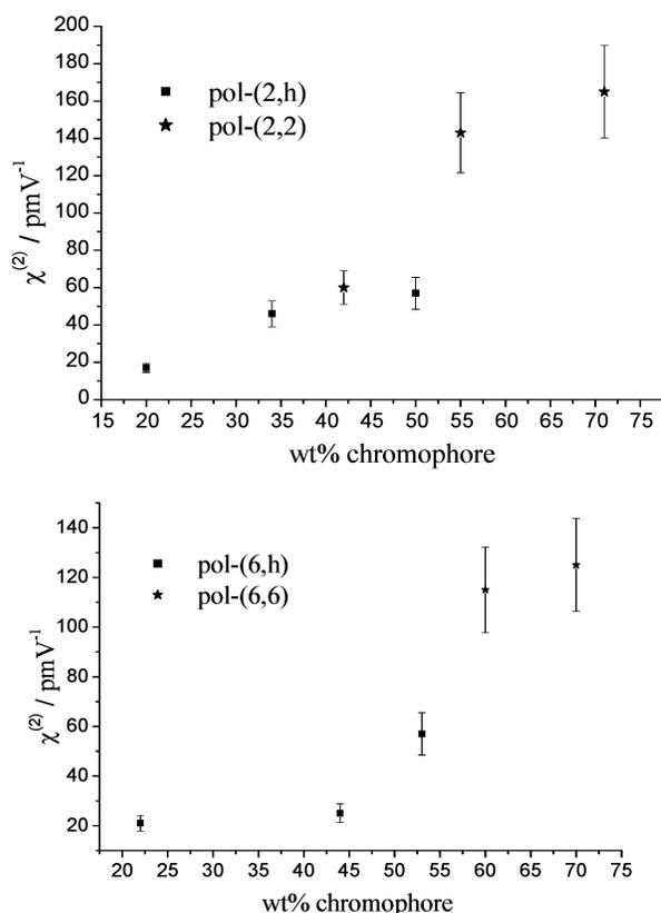
**Figure 4.** Evolution of  $\chi^{(2)}$  of the chromophore-functionalized polybinaphthalenes with increasing chromophore loading densities.
