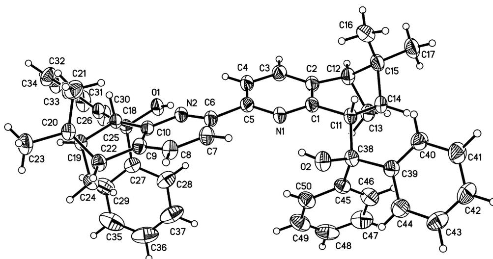
**Figure 2.** X-ray crystallographic structures of bipyridyldiol **6** (CCDC 757403).
