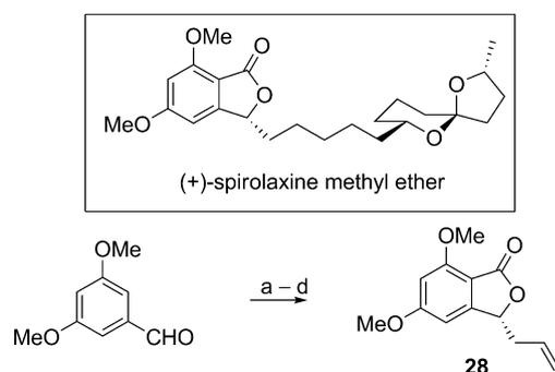
**Scheme 1.** Reaction conditions: a) Br<sub>2</sub>, AcOH; b) HOCH<sub>2</sub>CH<sub>2</sub>OH, *p*-TSA, benzene; c) *n*-BuLi, EtOCOCi; HCl; d) ligand **4a**, NH allylation.
