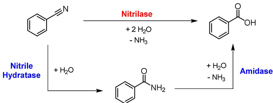
Figure 1. Enzymatic conversion of benzonitrile to the corresponding carboxylic acid (benzoic acid) and/or carboxamide (benzamide).
