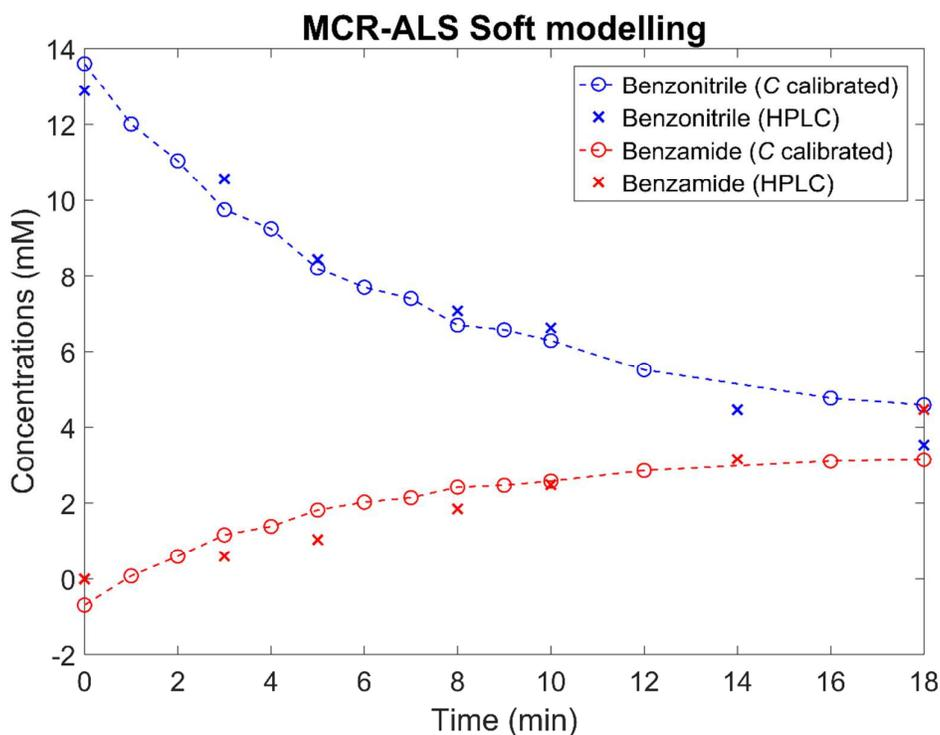
Figure 5. MCR-ALS model applied to the whole-cell biotransformation of benzonitrile (SM, blue) to benzamide (P, red) using NHase-containing *E. coli* cells. Figure shows the reaction dynamics from the real-time UVRr measurements (denoted by circular symbols) and off-line HPLC data (denoted by cross symbols) as a function of time.
