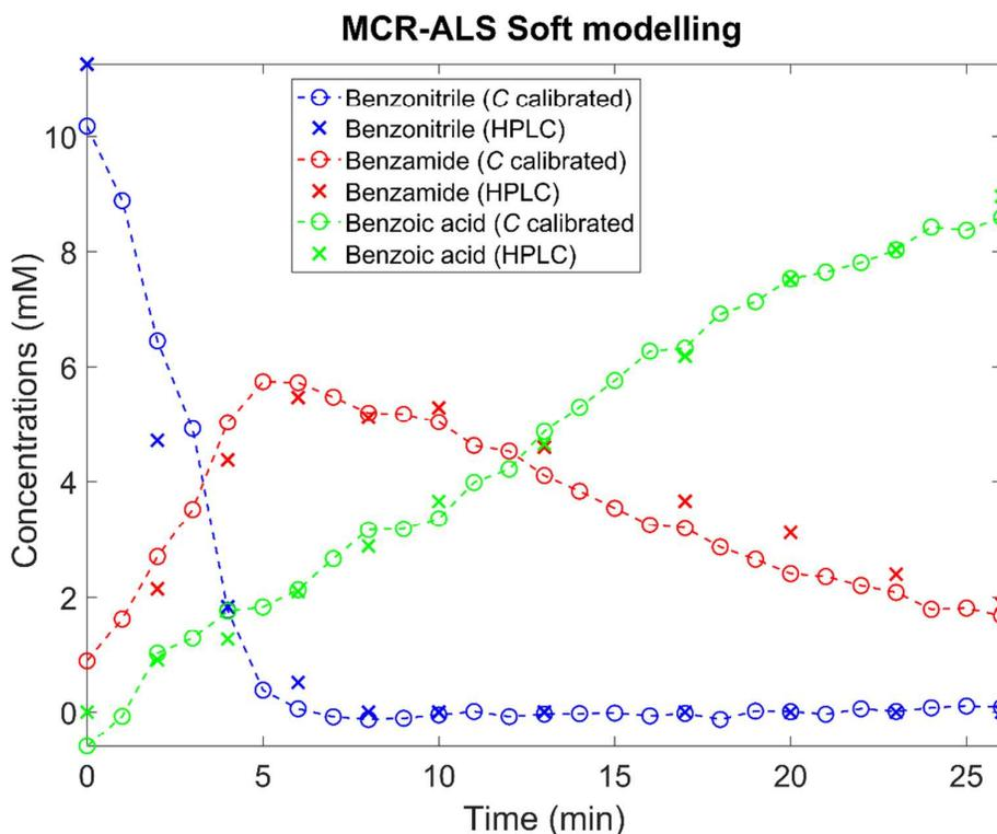
Figure 3. An MCR-ALS model was applied to the UVRR data where it successfully deconvolved spectra into its pure components for the biotransformation using pure enzymes. This figure shows the reaction dynamics from the real-time UVRR measurements (denoted by circular symbols) and off-line HPLC data (denoted by cross symbols) as a function of time for the conversion of benzonitrile (SM; blue) to benzamide (I; red) to benzoic acid (P; green), catalysed by NHase and amidase, correspondingly.
