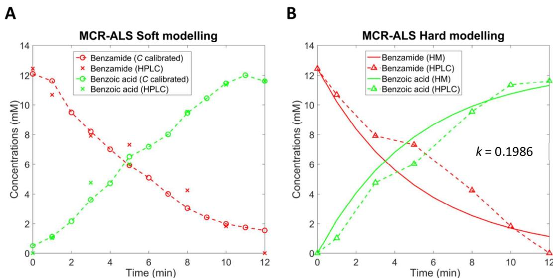
Figure 6. Modelling results for amidase-expressing bacterial whole-cells catalysing the conversion of benzamide (SM) to benzoic acid (P). **(A)** MCR-ALS soft modelling results and **(B)** MCR-ALS hard modelling results, kinetic rate was calculated as  $k = 0.1986$ .
