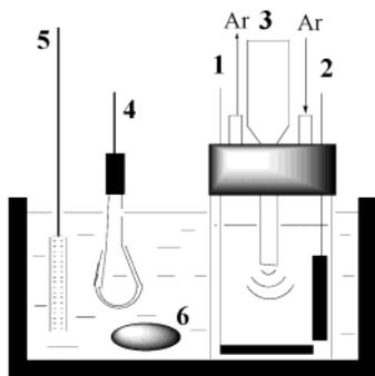
**Figure 1.** Apparatus for electro-synthesis under ultrasonic irradiation. Sonoelectrochemical system using a stepped horn: (1) working electrode (Pt 2 × 2 cm<sup>2</sup>), (2) counter electrode (Pt 2 × 2 cm<sup>2</sup>), (3) ultrasonic horn, (4) heater, (5) pipe-type cooler, (6) stirring bar.
