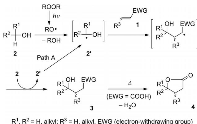
Scheme 1. Photochemical addition of alcohols to olefins.
