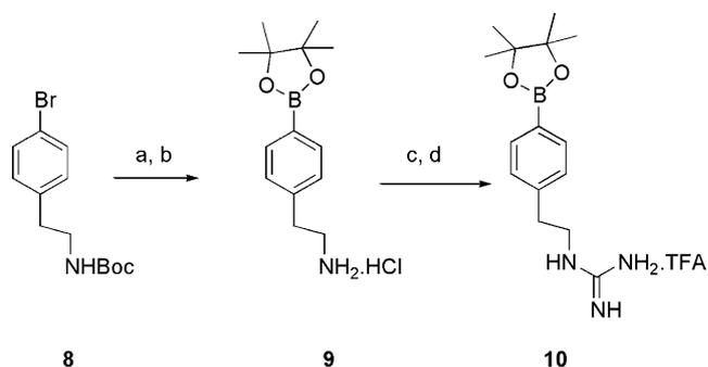
**Scheme 2.** Reagents and conditions: (a) 1 equiv dipinacolato diboron, 3 equiv KOAc, 0.1 equiv Pd(dppf)Cl<sub>2</sub>, DMSO, 80 °C, 18 h, 67%; (b) 4 N HCl, rt, 30 min, 96%; (c) 1 equiv **6**, 1 equiv *i*-Pr<sub>2</sub>EtN, DMF, rt, 18 h, 88%; (d) TFA, rt, 5 h, 94%.
