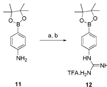
**Scheme 3.** Reagents and conditions: (a) 1 equiv **6**, 1 equiv *i*-Pr<sub>2</sub>EtN, DMF, rt, 18 h, 86%; (b) TFA, rt, 5 h, 90%.
