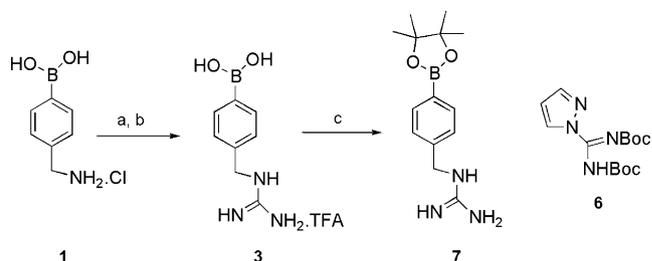
**Scheme 1.** Reagents and conditions: (a) 1 equiv **6**, 1 equiv *i*-Pr<sub>2</sub>EtN, DMF, rt, 18 h, 90%; (b) TFA, rt, 5 h, 87%; (c) 1 equiv pinacol, 1 equiv *i*-Pr<sub>2</sub>EtN, dioxane, 60 °C, 18 h, 91%.
