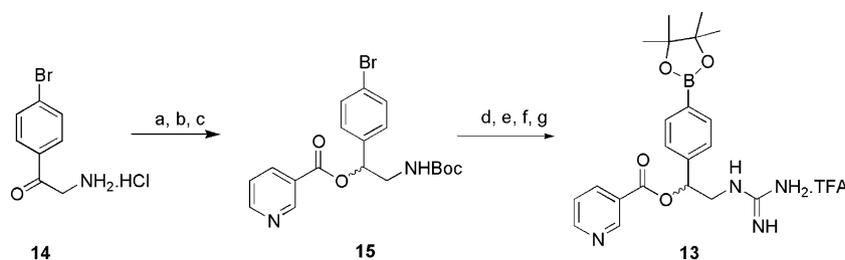
**Scheme 4.** Reagents and conditions: (a) 1.0 equiv (Boc)<sub>2</sub>O, 2.5 equiv Et<sub>3</sub>N, DCM, rt, 18 h, 96%; (b) 5 equiv NaBH<sub>4</sub>, methanol, rt, 1 h, 83%; (c) 1.0 equiv nicotinoyl chloride, 3 equiv *i*-Pr<sub>2</sub>EtN, DCM, rt, 18 h, 76%; (d) 1 equiv dipinacolato diboron, 3 equiv KOAc, 0.1 equiv Pd(dppf)Cl<sub>2</sub>, DMSO, 80 °C, 18 h, 73%; (e) 4 N HCl, rt, 30 min, 97%; (f) 1 equiv **6**, 1 equiv *i*-Pr<sub>2</sub>EtN, DMF, rt, 18 h, 85%; (g) TFA, rt, 5 h, 92%.
