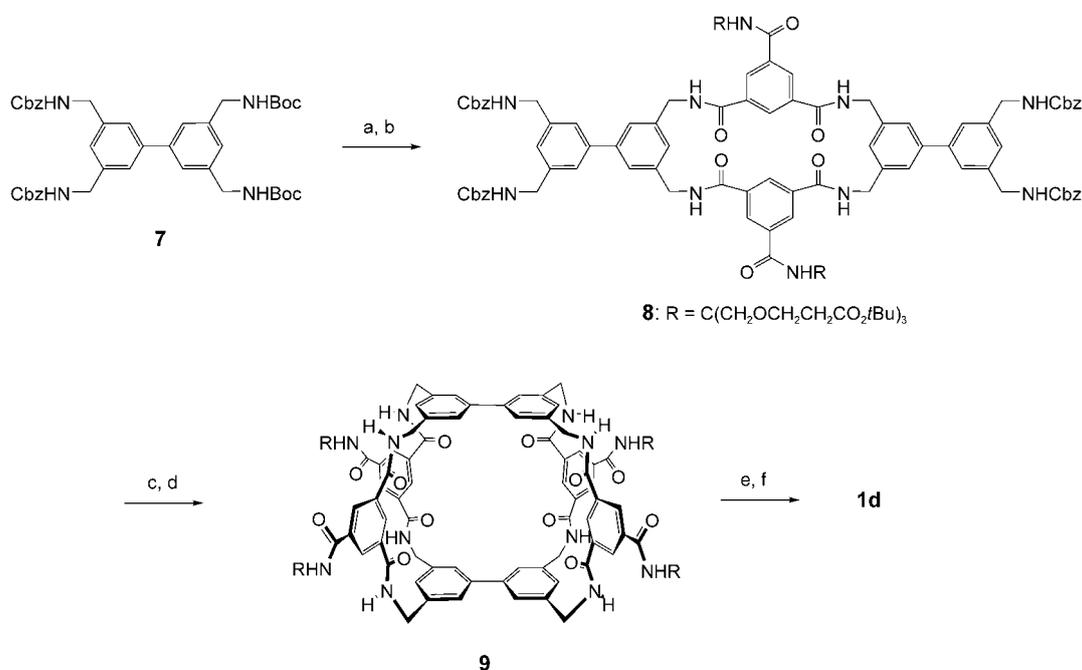
**Scheme 2.** Synthesis of **1d**: a) TFA, CH<sub>2</sub>Cl<sub>2</sub>; b) **6**, *i*Pr<sub>2</sub>NEt, THF, high dilution; c) H<sub>2</sub>, 10% Pd/C, THF/methanolic ammonia (1:1); d) **6**, *i*Pr<sub>2</sub>NEt, THF, high dilution; e) TFA, CH<sub>2</sub>Cl<sub>2</sub>; f) aq. NaOH (1 M). Boc = *tert*-butoxycarbonyl, Cbz = benzyloxycarbonyl, TFA = trifluoroacetic acid.
