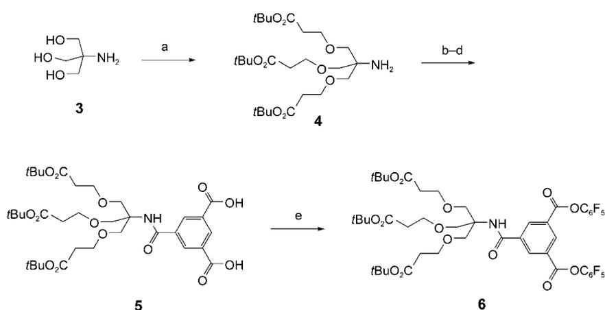
**Scheme 1.** Synthesis of **6**: a) *tert*-butyl acrylate, NaOH, DMSO, H<sub>2</sub>O; b) 1,3,5-benzenetricarbonyl trichloride (excess), *i*Pr<sub>2</sub>NEt, THF; c) aq. NaOH (2 M); d) aq. HCl (3.5 M); e) C<sub>6</sub>F<sub>5</sub>OH, DCC, THF. DMSO = dimethylsulfoxide, DCC = *N,N'*-dicyclohexylcarbodiimide.
