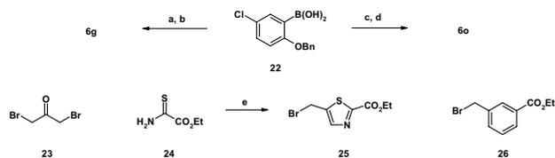
**Scheme 4.** Reagents and conditions: (a) **25**,  $Pd(PPh_3)_4$ ,  $K_2CO_3$ , PhMe–EtOH, 90 °C; (b) NaOH, EtOH  $H_2O$ , 60 °C, 2 h; (c) **26**,  $Pd(PPh_3)_4$ ,  $Na_2CO_3$ ,  $H_2O$ , DME–EtOH, 90 °C; (d) 2 M NaOH, EtOH, reflux; (e) EtOH, reflux, 15 h.
