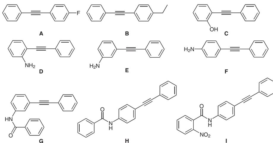
Figure 3 Control experiments to prove the amide is a directing group: no reaction in all cases (**A–I**)
