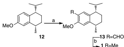
**Scheme 4.** Synthesis of *cis*-7-methoxy-calamenene **1**, reagents and conditions: (a)  $P_2O_5Cl_4$ , DMF,  $0^\circ C$  to reflux, 24 h, 56%; (b)  $H_2$ , Pd/C, MeOH, 3 h, 99%.
