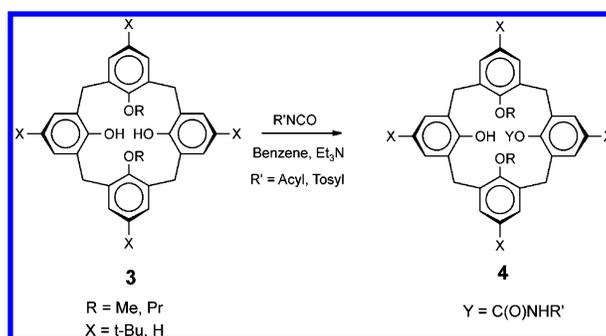
Calix[4]arenedialkyl ethers **3** react with an excess of acylisocyanates to give selectively monoacylated products **4**. Intramolecular hydrogen bonds and steric effects of the acylcarbamate fragments are most likely responsible for the high selectivity of this monoprotection.
