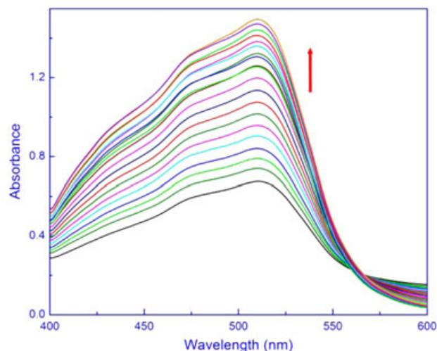
**Figure 2.** Increase in the absorbance of  $[\text{Fe}(\text{phen})_3]^{3+}$  during the reaction with the isobestic point
