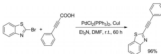
Scheme 2. Pd-catalyzed coupling of **1a** with phenylpropionic acid.
