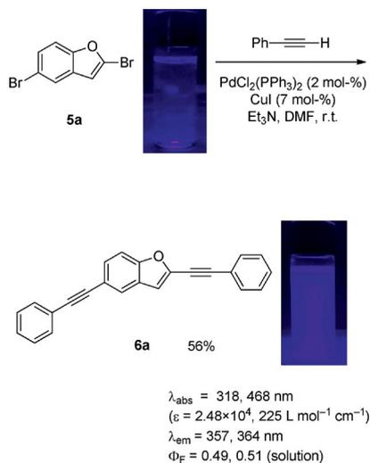
Scheme 3. The fluorescence of 2,5-bis(2-phenylethynyl)benzofuran.
