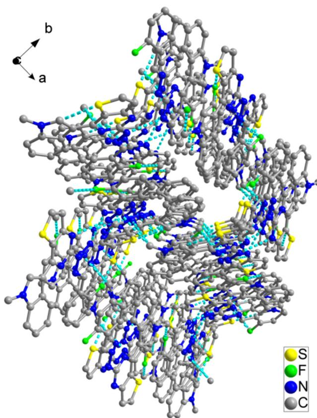
**Figure 2.** A packing diagram of the title compound ( $C_{22}H_{16}FN_5S$ ).
