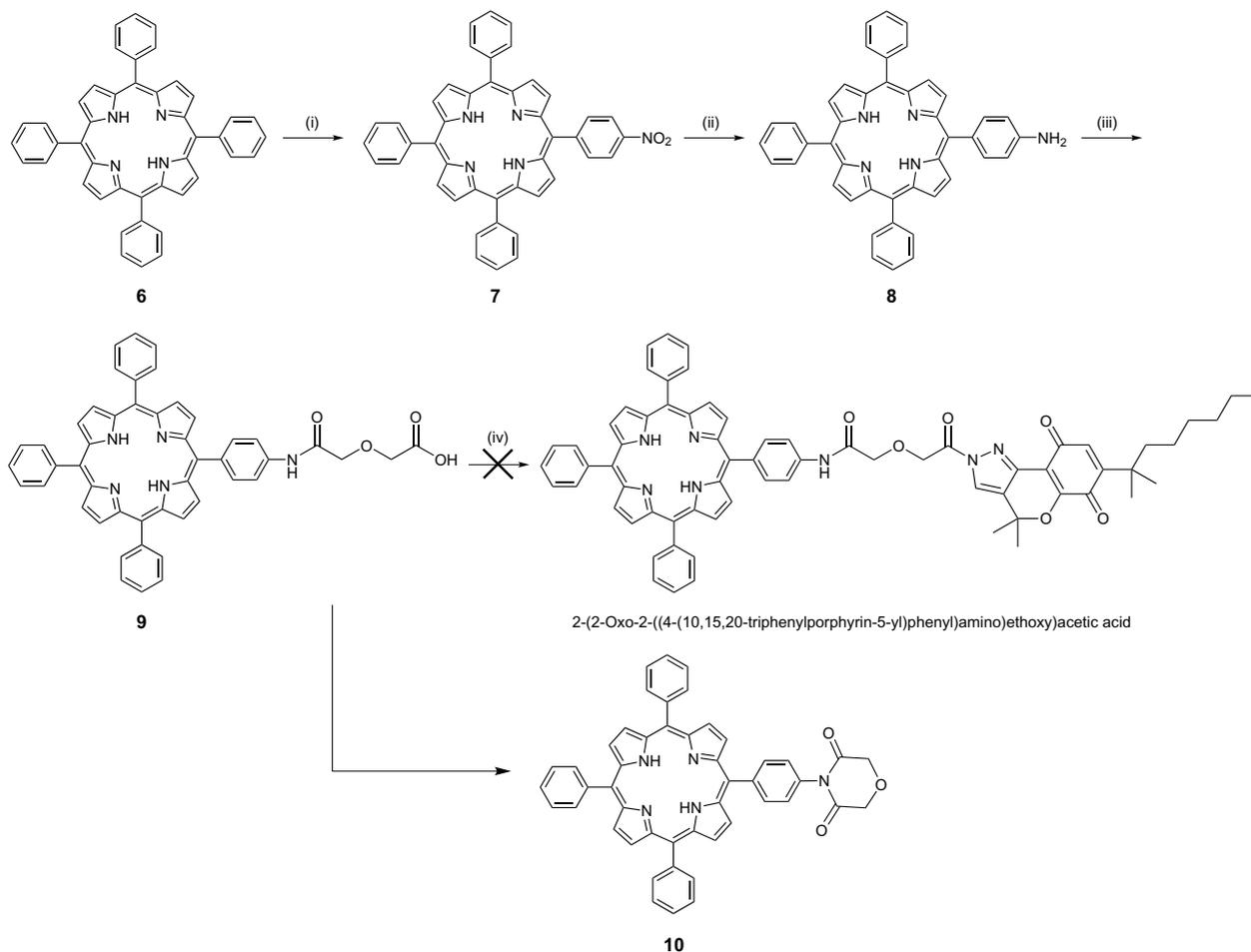
**Scheme 2.** Synthesis of porphyrin derivatives. Reaction conditions. (i) NaNO<sub>2</sub> (1.8 equiv), TFA, 25 °C, 3 min (49%). (ii) SnCl<sub>2</sub>, conc. HCl, 65 °C, 1 h (96%). (iii) Diglycolic anhydride, DMF, rt, 24 h (85%). (iv) (a) SOCl<sub>2</sub>, toluene, 120 °C, 30 min, MW; (b) chromenopyrazole **5**, NaH, CH<sub>2</sub>Cl<sub>2</sub>, rt, overnight
