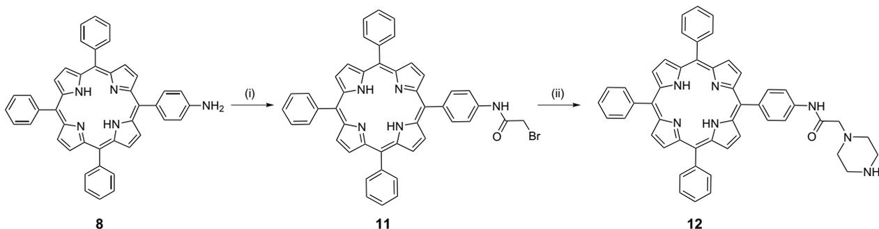
**Scheme 3.** Synthesis of the porphyrin-piperazine intermediate **12**. Reaction conditions. (i) Bromoacetyl bromide, Et<sub>3</sub>N, CH<sub>2</sub>Cl<sub>2</sub>, 25 °C, 1 h (31%). (ii) Piperazine, CH<sub>2</sub>Cl<sub>2</sub>, 25 °C, 45 min (96%)
