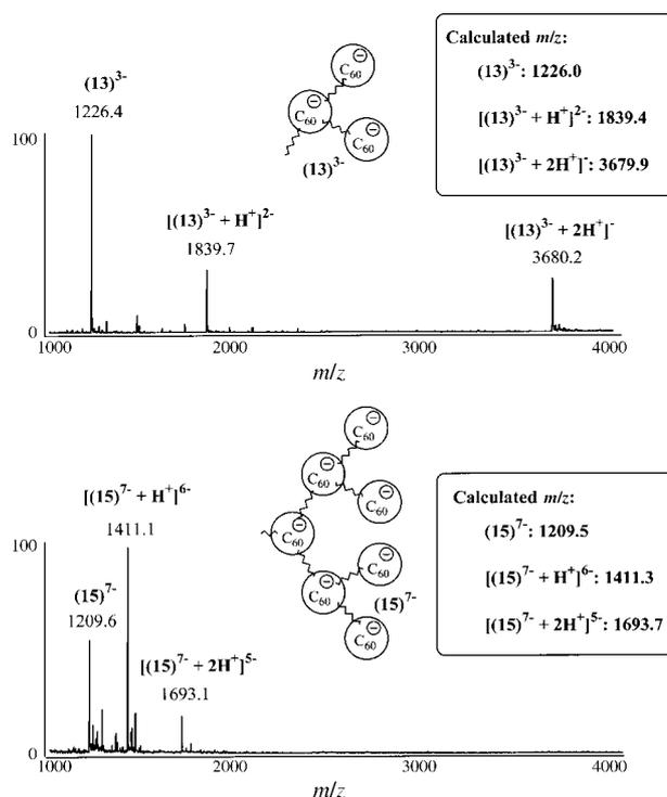
Fig. 4 ES mass spectra of **13** (top) and **15** (bottom).
