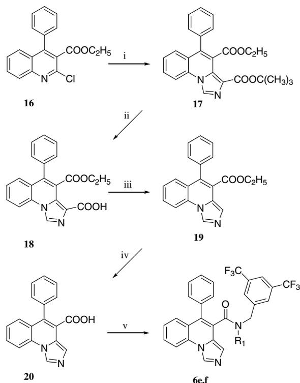
**Scheme 3.** Reagents: (i) *tert*-Butyl isocyanacetate, *t*-BuOK, DMF; (ii) HCOOH; (iii) Δ, no-solvent (neat), N<sub>2</sub>; (iv) NaOH, C<sub>2</sub>H<sub>5</sub>OH; (v) 3,5-(CF<sub>3</sub>)<sub>2</sub>C<sub>6</sub>H<sub>3</sub>CH<sub>2</sub>NH<sub>2</sub>, HOBT, DCC, CH<sub>2</sub>Cl<sub>2</sub> or 3,5-(CF<sub>3</sub>)<sub>2</sub>C<sub>6</sub>H<sub>3</sub>CH<sub>2</sub>N(H)CH<sub>3</sub>·HCl, HOBT, DCC, TEA, CH<sub>2</sub>Cl<sub>2</sub>.
