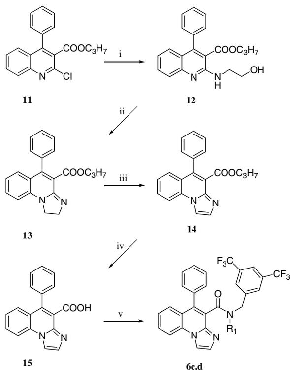
**Scheme 2.** Reagents: (i) HOCH<sub>2</sub>CH<sub>2</sub>NH<sub>2</sub>, C<sub>2</sub>H<sub>5</sub>OH; (ii) POCl<sub>3</sub>; (iii) Δ, DMSO; (iv) NaOH, C<sub>2</sub>H<sub>5</sub>OH; (v) 3,5-(CF<sub>3</sub>)<sub>2</sub>C<sub>6</sub>H<sub>3</sub>CH<sub>2</sub>NH<sub>2</sub>, HOBT, DCC, CH<sub>2</sub>Cl<sub>2</sub> or 3,5-(CF<sub>3</sub>)<sub>2</sub>C<sub>6</sub>H<sub>3</sub>CH<sub>2</sub>N(H)CH<sub>3</sub>·HCl, HOBT, DCC, TEA, CH<sub>2</sub>Cl<sub>2</sub>.
