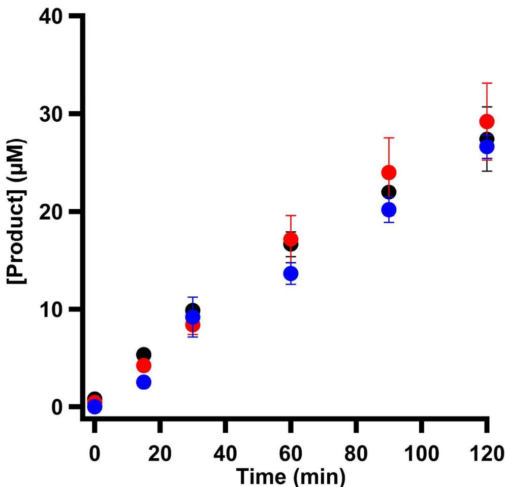
**Figure 7.** Time-dependent formation of HPP-CMP (black), SAH (red), and 5'-dA (blue) by Fom3 ( $9 \mu\text{M}$ ) in the presence of  $1.5 \text{ mM}$  HEP-CMP,  $1.5 \text{ mM}$  SAM,  $1 \text{ mM}$  methyl viologen and  $2 \text{ mM}$  NADPH.
