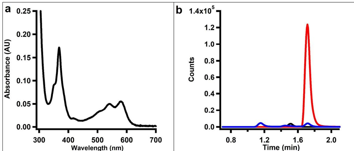
**Figure 8.** (a) UV-Vis spectrum of PhpK (6.5  $\mu$ M) treated with potassium cyanide. (b) LC-MS/MS analysis of as-isolated PhpK, which contains 8% AdoCbl (black), 15% OHCbl (blue), and 77% MeCbl (red).
