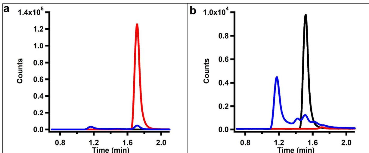
**Figure 6.** LC-MS/MS analysis of the cobalamin content of (a) as-isolated Fom3 (20  $\mu$ M) and (b) as-isolated TsrM. (a) As-isolated Fom3 contains 18% OHCbl (blue line), 0% AdoCbl (black line) and 82% MeCbl (red line). (b) TsrM contains 61% OHCbl (blue line), 39% AdoCbl (black line) and <1% MeCbl (red line).
