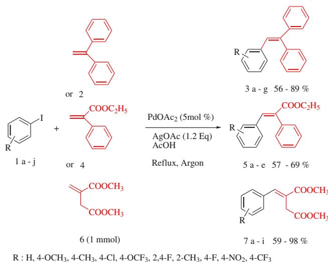
**SCHEME 1** Pd(OAc)<sub>2</sub> (cat)/AgOAc mediated Mizoroki-Heck reaction with 1, 1 -disubstituted alkenes<sup>a</sup>
