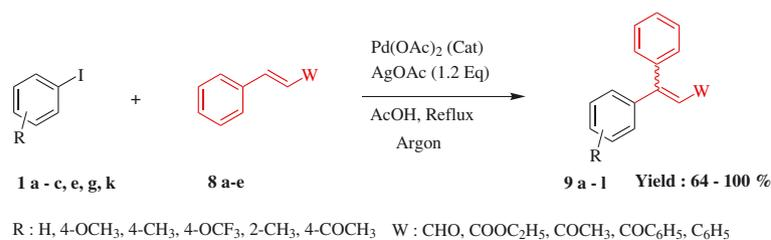
**SCHEME 2** Pd(OAc)<sub>2</sub> (Cat)/AgOAc mediated Mizoroki-Heck reaction of 1,2-disubstituted alkenes<sup>a</sup>
