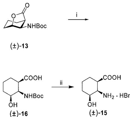
Scheme 3. Reagents and conditions: (i) LiOH, H<sub>2</sub>O, THF, room temp., 5 h, 98%; (ii) Me<sub>3</sub>SiBr, phenol, CH<sub>2</sub>Cl<sub>2</sub>, room temp., 2 h, Ar atmosphere, 76%.
