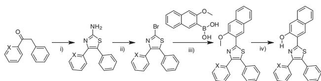
**Scheme 2.** Synthetic routes for the ESIPT-based chemosensor molecules.
