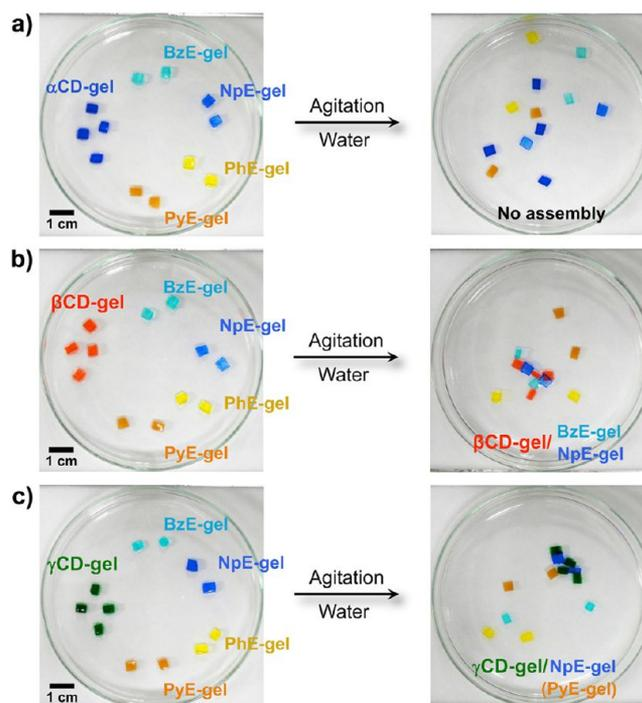
**Figure 2.** Pictures of the interaction of  $\alpha$ CD-gel (gentian blue) (a),  $\beta$ CD-gel (red) (b), and  $\gamma$ CD-gel (bottle green) with the ArE-gels {BzE-gel (sky blue), NpE-gel (blue), PhE-gel (yellow), and PyE-gel (orange)} (c).
