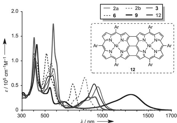
**Figure 3.** UV/Vis/NIR absorption spectra of **2a**, **2b**, **3**, **6**, **9**, and **12** in  $\text{CH}_2\text{Cl}_2$ .  $\lambda$  = wavelength,  $\epsilon$  = extinction coefficient, Ar = 3,5-di-*tert*-butylphenyl.
