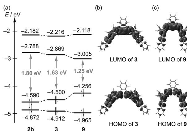
**Figure 4.** a) Energy diagrams of the HOMO and LUMO of b) **3** and c) **9**. All of the calculations were performed at the B3LYP/6-31G(d) (for C,H,N) + LANL2DZ (for Ni) level. *tert*-Butyl groups were replaced to hydrogen atoms to simplify the calculations.
