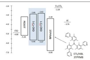
Scheme 2. Energy level diagram of the OLED devices and molecular structure of 3TPYMB
