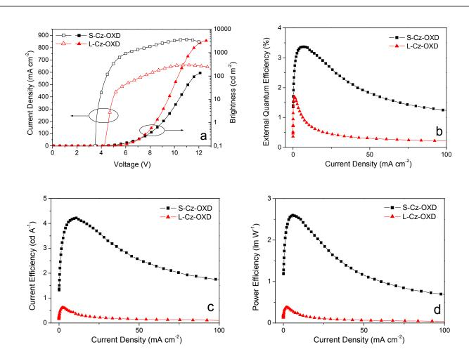
Figure 5.(a) Current density-voltage and brightness-voltage spectra of devices; (b) Current efficiency versus current density of devices; (c) Power efficiency versus current density of devices; (d) External quantum efficiency versus current density of devices.
