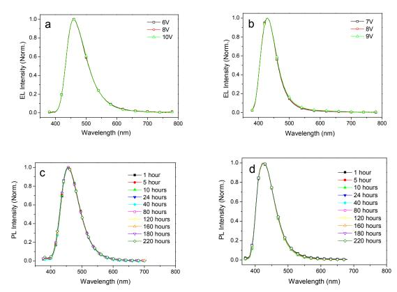
Figure 4.Normalized EL spectra of devices based on (a) S-Cz-OXD and (b) L-Cz-OXD at different applied voltages, and PL spectra of (c) S-Cz-OXD and (d) L-Cz-OXD during heating process at 150 °C in ambient air
