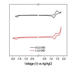
Figure 2. Cyclic voltammograms of S-Cz-OXD and L-Cz-OXD
