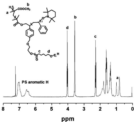
**Figure 8.**  $^1\text{H}$  NMR spectrum of a star terpolymer composed of poly( $\epsilon$ -caprolactone), poly(methyl methacrylate), and polystyrene arms (CMS-3 in Table 2).
