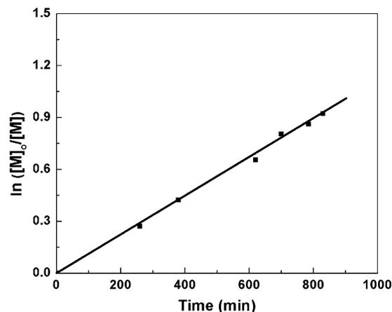
**Figure 3.** Relationship between  $\ln([\text{M}]_0/[\text{M}])$  and the polymerization time in the ring-opening polymerization of  $\epsilon$ -caprolactone using trifunctional initiator 5 and  $\text{Et}_3\text{Al}$  as the initiation system in toluene at room temperature.  $[\text{M}]_0/[\text{I}]_0 = 135$ ;  $[\text{I}]_0/[\text{AlEt}_3]_0 = 1:1.05$ .
