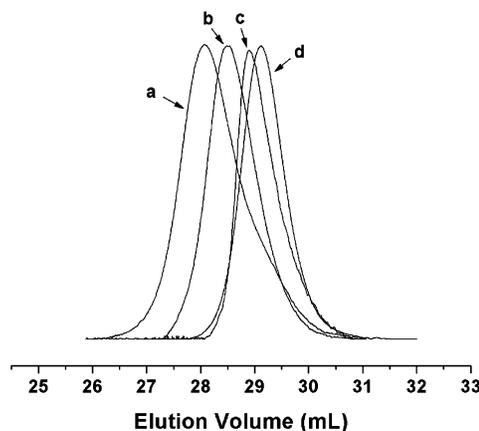
**Figure 9.** GPC analysis of the polymers obtained in arm cleavage experiments: (a) a star terpolymer (CMS-2); (b) the polymer obtained after reaction for 4 h; (c) poly(methyl methacrylate) obtained after reaction for 4 days and removal of polystyrene by extraction with cyclohexane for 3 h; (d) polystyrene obtained after reaction for 4 days and extraction with cyclohexane for 3 h.
