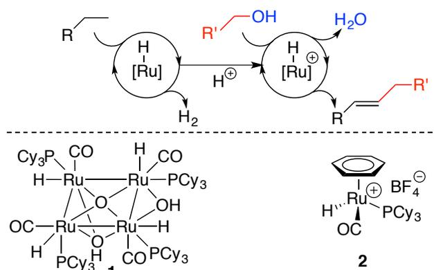
**Scheme 1. General Tandem Dehydrogenation-Alkylation Reaction Scheme and the Structure of Ruthenium Catalysts.**
