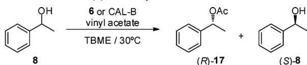
*rac*-1-phenylethanol (**8**) with vinyl acetate (3 equiv) in TBME at  $30\text{ }^{\circ}\text{C}$  (Scheme 6) to achieve the kinetic resolution of this substrate. We confirmed that immobilized CAL-B was able to perform this reaction with high selectivity ( $c = 49\%$ ), affording both enantiopure substrate and product after 24 h. Interestingly, under the same conditions, commercial pure CAL-B afforded a conversion of 17%, evidencing an important stability enhancement for this lipase.
