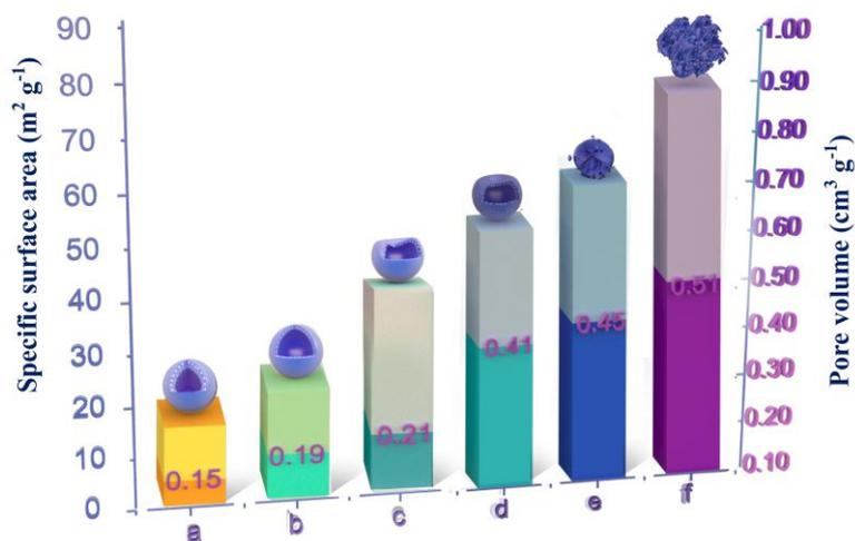
**Fig.6.** Architectural features of various catalysts: (a) PS-NH<sub>2</sub> OPNs, (b) PS-NH<sub>2</sub> HOPNs, (c) PS-NH<sub>2</sub> HMOPBs, (d) #PS-NH<sub>2</sub> HMOPBs(80), (e) #PS-NH<sub>2</sub> HMOPBs(115), and (f) #PS-NH<sub>2</sub> HMOPBs(145).
