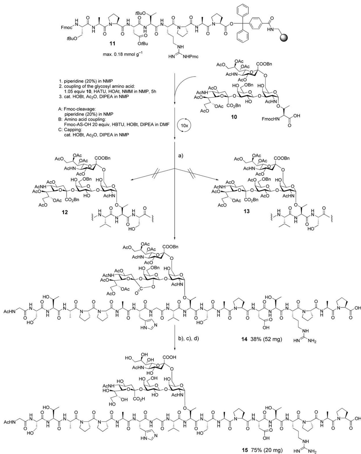
**Scheme 2.** a) TFA, TIS, H<sub>2</sub>O (15:0.9:0.9); b) H<sub>2</sub>, Pd/C (10%), MeOH; c) NaOMe/MeOH, pH 9.5; d) NaOH (aq), pH 11.5, 1 h; then AcOH. DIPEA = diisopropylethylamine.
