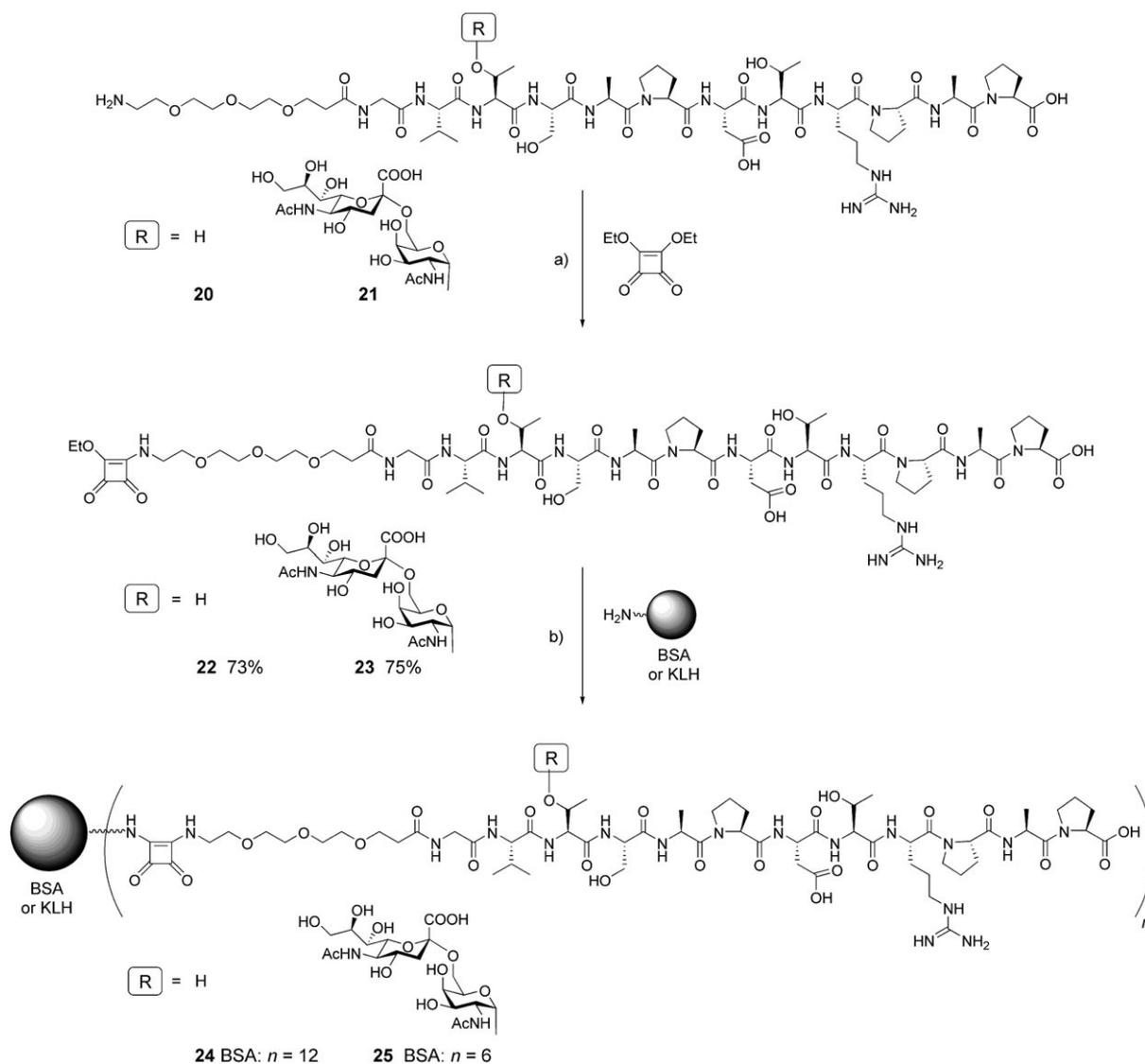
**Scheme 4.** a) Ethanol/water (1:1),  $\text{Na}_2\text{CO}_3$ , pH 8.0, 2 h, preparative HPLC; b) sodium borate (0.07 M),  $\text{NaHCO}_3$  (0.035 M), pH 9, 24 h, gel filtration chromatography (Sephadex-G25 PD10 column), dialysis against  $\text{H}_2\text{O}$ .
