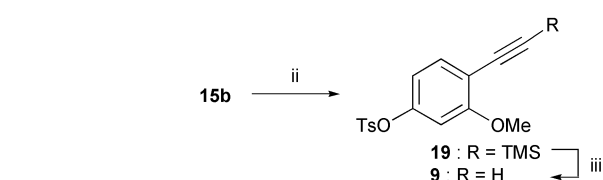
Scheme 6 Reagents, conditions and yields: i, KI, CuI, HMPA, 150 °C, 94% (15a → 15b), 94% (8a → 8b); ii, trimethylsilylacetylene, PdCl 2 (PPh 3 ) 2 , CuI, Et 3 N, DMF, RT, 98%; iii, TBAF, THF, RT, 99%.
