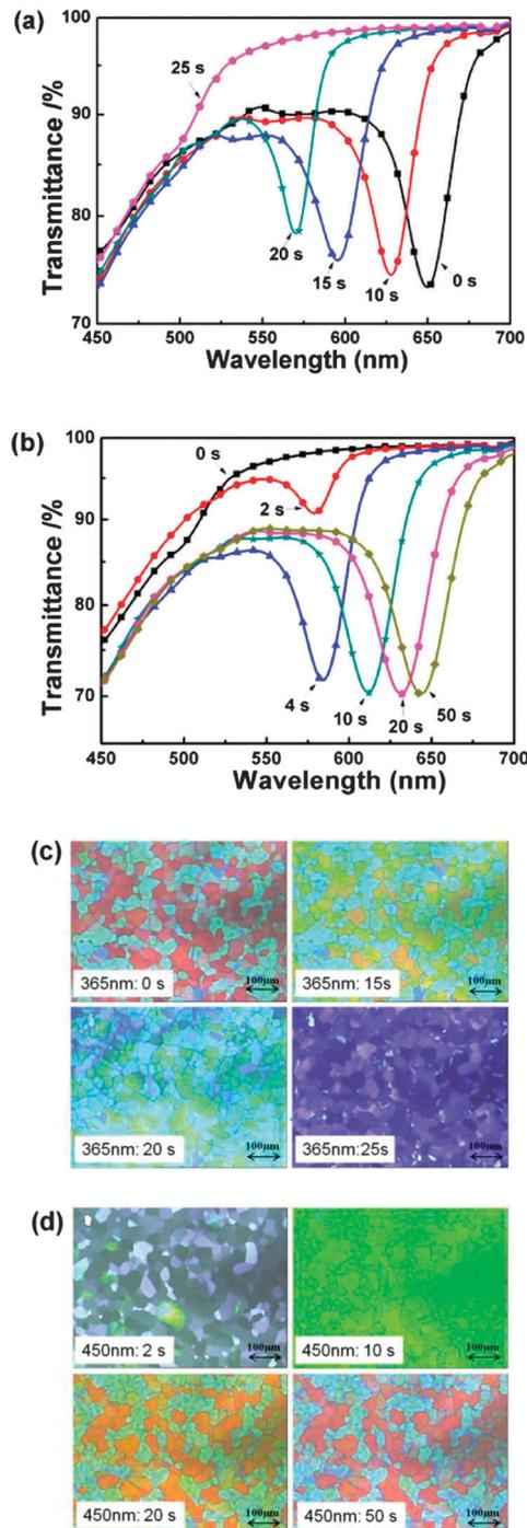
**Fig. 2** (a) The transmittance spectral change of the composite A1 when irradiated by UV at 38.5 °C; (b) the transmittance spectral change of A1 when irradiated by visible light after irradiation by UV; (c) change in POM pictures of the composite A1 when irradiated by UV at 38.5 °C; (d) POM picture of A1 irradiated by visible light after irradiation by UV.
