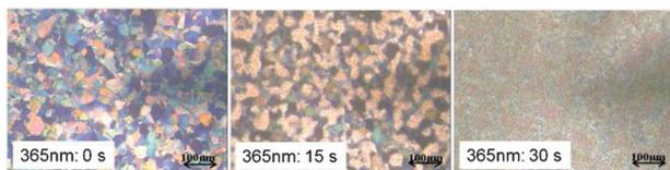
**Fig. 4** POM pictures of A3 irradiated by UV at 35 °C.
