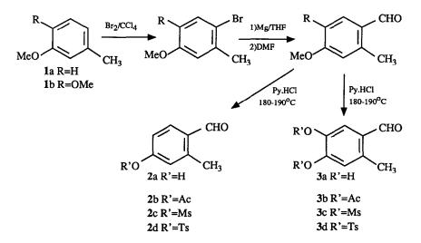
The irradiation of the acetate 2b (from 2a,  $Ac_2O/NaOAc$ , r. temp, under  $N_2$ , 96%) in benzene/SO<sub>2</sub>(10% SO<sub>2</sub> by weight, medium pressure mercury lamp through 1 mm pyrex) gave a slow decomposition of the starting material but we were unable to isolate the sulfone adduct 4b.
