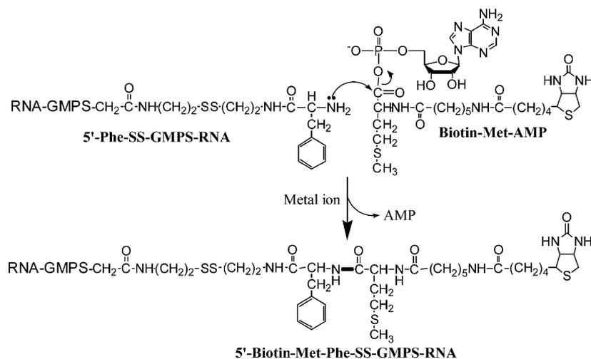
**Figure 1.** The peptide bond-forming reaction of biotin-Met-adenylate with 5'-Phe-SS-GMPS-RNA.
