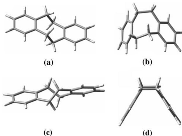
**Fig. 1** Optimized ground state structures of the **a** chair (C), **b** twist-boat (TB), **c** twist (T), and **d** boat (B) conformations of THDC. The boat conformation corresponds to a transition state between two equivalent TB conformers
