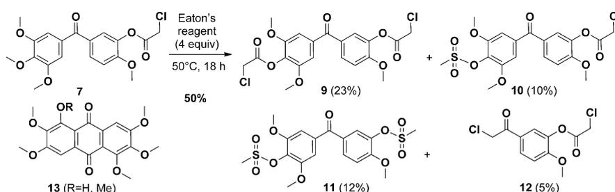
**Scheme 2.** Results of the evolution of phenstatin precursor **7** in Eaton's reagent under the optimized reaction conditions.
