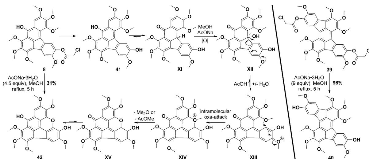
**Scheme 7.** Cleavage of the chloroacetyl protecting group of benzo[*a*]aceanthrylene **8** and rubicene **39** PAH derivatives and a corresponding plausible mechanistic scheme.
