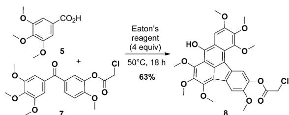
**Scheme 3.** Reaction of phenstatin precursor **7** with trimethoxybenzoic acid (**5**) leading solely to red product **8**.
