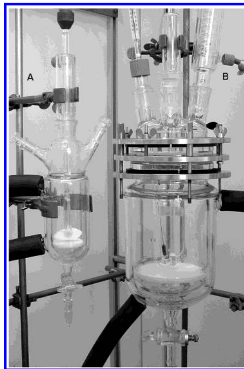
Figure 4. Reactors with coarse fritted filter plates: (A) 250 mL, equipped with three-necks, jacket, and mechanical glass stirrer with Teflon paddle and (B) 1.5 L, equipped with jacket, glass anchor stirrer, and a five-necked clamped top.
