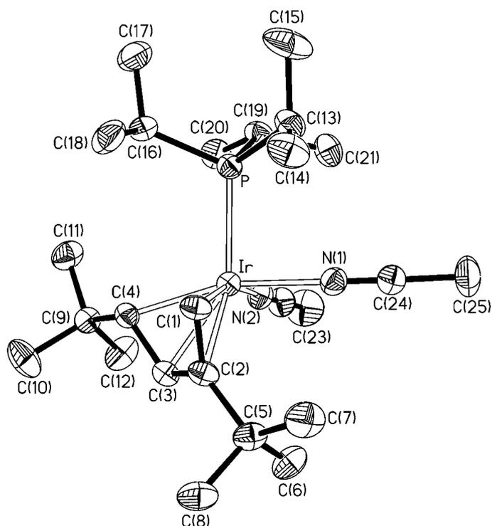
**Figure 1.** Molecular structure of the cation of complex **5** (ORTEP). Selected bond distances [Å] and angles [°]: Ir–P 2.3559(12), Ir–N1 2.1000(4), Ir–N2 2.090(4), Ir–C1 2.111(4), Ir–C2 2.193(4), Ir–C3 2.179(4), Ir–C4 2.151(4); C1–C2–C3 113.3(4), C2–C3–C4 118.6(4), C3–C4–C9 118.1(4).
