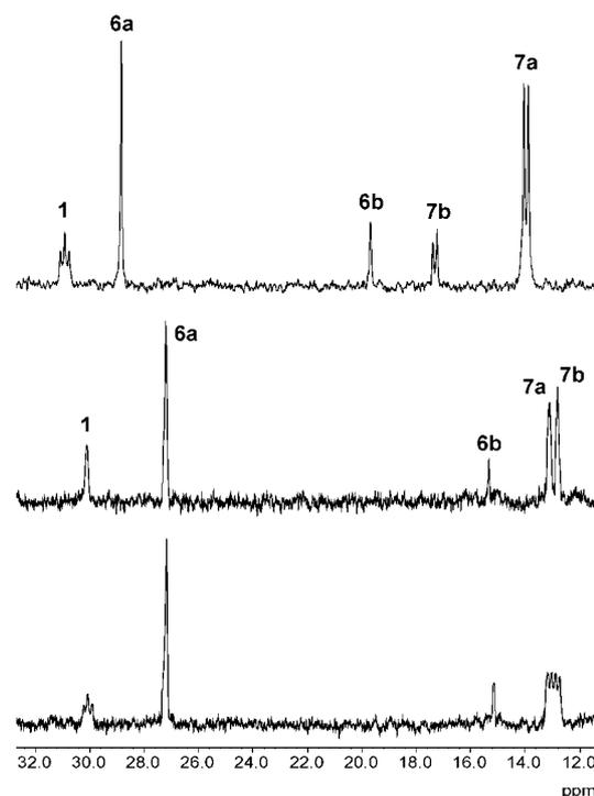
**Figure 3.** <sup>31</sup>P NMR spectra of compound mixtures obtained by treatment of **1** with PhC≡CH at room temperature: (above) <sup>31</sup>P off resonance spectrum in CDCl<sub>3</sub>; (center) <sup>31</sup>P{<sup>1</sup>H} spectrum in BMIM·BF<sub>4</sub>; (below) <sup>31</sup>P off resonance spectrum in BMIM·BF<sub>4</sub>.
