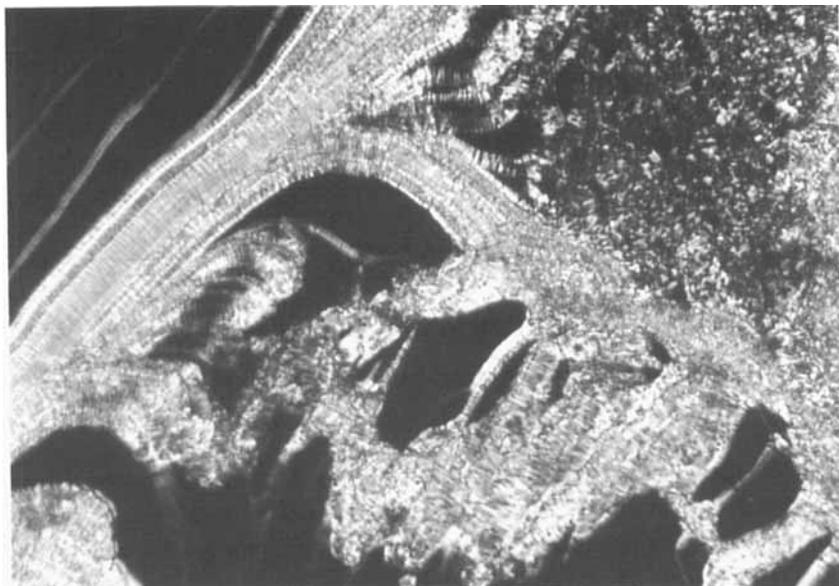
FIGURE 3 The characteristic oily streak pattern of the  $S_A$  phase of C16MO at 120°C formed on heating the crystal (at the rate of 10°C/min) (See Color Plate III at the back of this issue)
