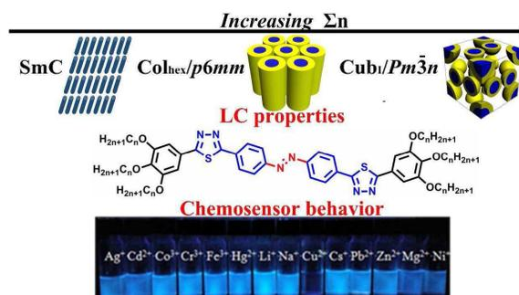
Target compounds can self-assemble into thermotropic LC phase sequence of SmC-Col<sub>hex</sub>-Cub<sub>1</sub>, and have binding selectivity to Cu<sup>2+</sup>.
