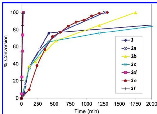
**Figure 1.** Relative rates of AROM/CM reactions (to afford **11a**) catalyzed by various chiral Ru catalysts (22 °C). (Reactions with catalysts **3** and **3c** require 4000 min to proceed to >98% conv).
