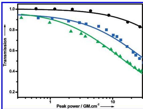
**Figure 2.** Nonlinear transmission of **stilbene-420** (black circle) reference in water, **10** (blue square), and **11** (green triangle) in  $\text{CH}_2\text{Cl}_2$  ( $c = 10^{-2} \text{ mol L}^{-1}$ ). The continuous lines are the best fit to a TPA law (see Supporting Information).
