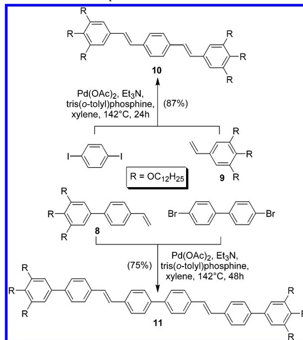
In this paper, we report on the synthesis of two hexacatenar molecules (mesogens with a long rigid core bearing three aliphatic chains at both extremities),<sup>10</sup> the OBV-3 **11** and the OPV analogue **10**, their one- and two-photon properties, and their thermal behavior.
