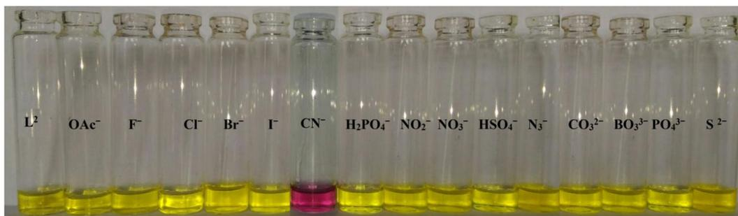
**Fig. 3.** Color changes of (a) **L**<sub>1</sub> and (b) **L**<sub>2</sub> after addition of 10 equiv. of different anions in CH<sub>3</sub>CN-H<sub>2</sub>O (2:1, v/v) mixture.
