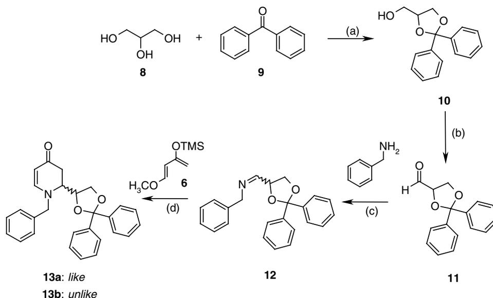
**Scheme 1.** Synthesis of dihydropyridones **13a/b** (all compounds are racemic). Reagents and conditions: (a) TosOH-H<sub>2</sub>O, toluene, reflux, 6 h, yield 73%; (b) oxalyl chloride, DMSO, CH<sub>2</sub>Cl<sub>2</sub>, -78 °C, 30 min, then NEt<sub>3</sub>, rt, yield 72%; (c) benzylamine, trimethyl orthoformate, rt, 16 h; (d) Yb(OTf)<sub>3</sub>, THF, 0 °C (4 h) then 25 °C (16 h), yield 70% from **11**.
