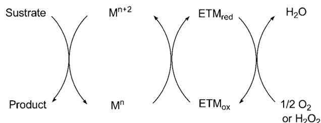
Scheme 1. Biomimetic oxidation involving electron-transfer mediator (ETM).
