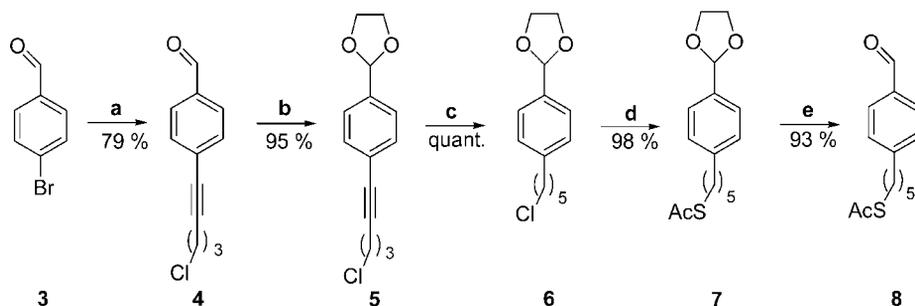
Scheme 2. Reagents and conditions: **a.** 5-chloro-1-pentyne,  $\text{Pd}(\text{OAc})_2$ ,  $\text{PPh}_3$ ,  $\text{NEt}_3$ ,  $\text{CuI}$ , THF, room temp. overnight; **b.** ethylene glycol,  $\text{TsOH}$ , benzene, reflux, 12 h; **c.**  $\text{RhCl}(\text{PPh}_3)_3$ ,  $\text{H}_2$ , benzene, room temp. 14 h; **d.**  $\text{KSAc}$ , reflux, 13 h,  $56^\circ\text{C}$ ; **e.**  $\text{TsOH}$ , acetone,  $\text{H}_2\text{O}$ , reflux, 14 h.
