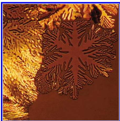
Figure 1. Polarized optical photomicrograph of monotropic phase of 3b at 158 °C (100× magnification).
